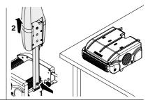
**3** Unhook the upper cover of the machine and wash it thoroughly with running water.
