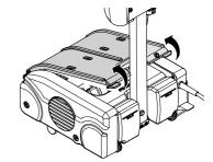
**2** Remove and empty the dirty water waste. Wash it with running water and, if necessary, use a spatula to remove any residual from the bottom.
