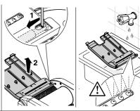
**4** Unhook and drain the clean water tank 2 from any residual of water and/or detergent.
