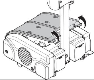
**2** Remove and empty the dirty water waste. Wash it with running water and, if necessary, use a spatula to remove any residual from the bottom.
