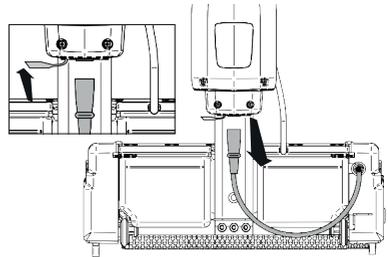
**2** Gently push the battery down and at the same time pull the release button towards you.
