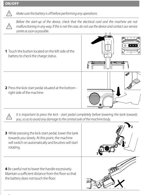
Do not press the kick - start pedal when returning the tank to the original position.
